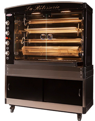
MAGFLAM 40/8 Gas only W: 43" D: 27" H: 77 1/2" (with cabinet) 24 to 32 chickens/hour 3 Burners - 112,000 BTU/hr (Natural Gas)
