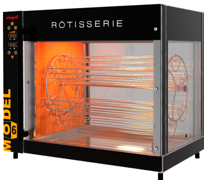
MODEL 6 Electric W: 40 1/2" D: 30 5/8" H: 37 3/4" 20 to 30 chickens/hour 220 V Triphase - 11.3 Kw - 30 Amps
